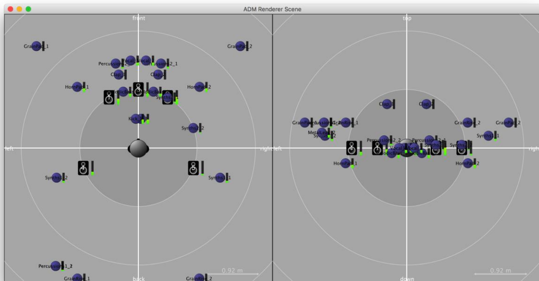
Figure 7: Scene display of the ADM Player/Renderer playing the file machine-aer_bwf.wav [5]. Left pane: view from above; Right pane: view from behind
