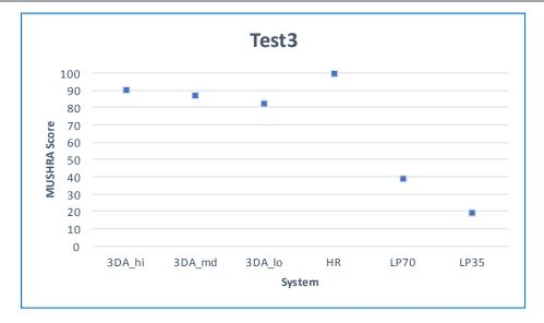
Figure 10: Test 3 "High Efficiency Broadcast". For formats and bitrates see Table 1. The size of the confidence interval is so small that it is within the size of the marker used for the mean<sup>18</sup>.
