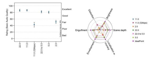
Figure 14: Overall system basic audio quality ratings for different loudspeaker reproduction setups; b) Spider plot of attribute rating with 95% confidence circles, from<sup>21</sup>
