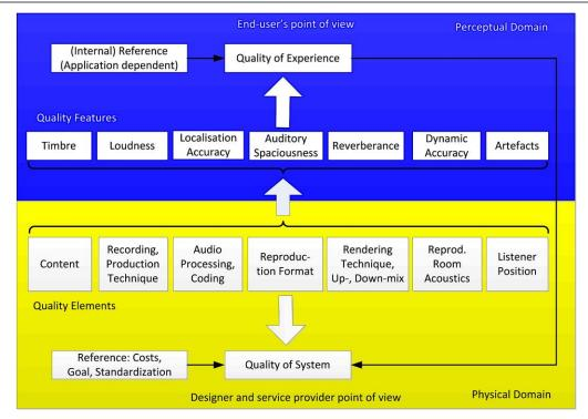
Figure 16: Quality Taxonomy for 3D audio systems, with the Quality Elements in the physical domain and the Quality Features in the perceptual domain. The Quality of Experience and the Quality of System are comparisons between their input parameters and the given references<sup>23</sup>
