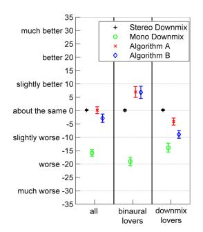
Figure 12: Using a bi-polar scale and cluster analysis for comparison of binaural renderers to a standard downmix of 5.1 items <sup>19</sup>
