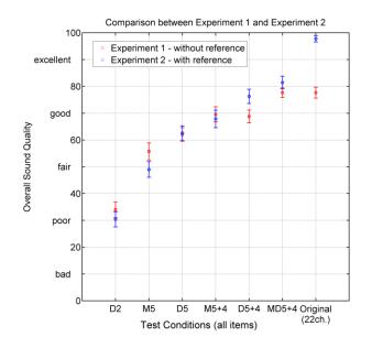
Figure 13: Comparison between different loudspeaker reproduction setups, with and without reference; x+y: x loudspeaker on ear height, y elevated loudspeakers, D downmix, M leaving out channels<sup>20</sup>
