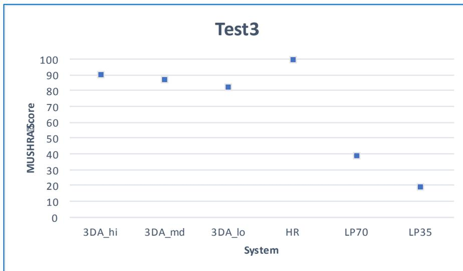
Figure 10: Test 3 "High Efficiency Broadcast". For formats and bitrates see Table 1. The size of the confidence interval is so small that it is within the size of the marker used for the mean<sup>18</sup>.
