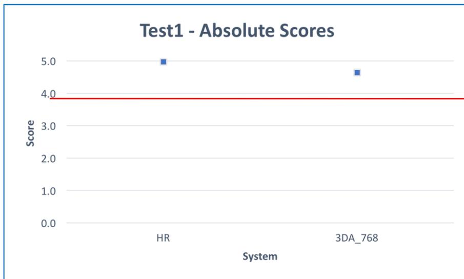
Figure 8: Test 1 “Ultra HD Broadcast”, HR hidden reference, 3DA\_768 3D audio material in 768 kbit/s, the red line shows the ITU-R requirement for “high-quality emission,” i.e. mean value of 4.0, The size of the confidence interval is so small that it is within the size of the marker used for the mean<sup>18</sup>.
